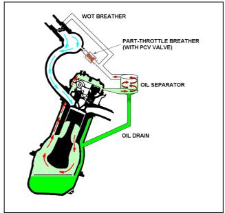
Figure 12: An external oil separator.
