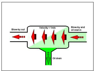
Figure 9: A simple oil separator volume.
