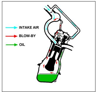
Figure 4: Low blow-by / low load breather flow.
