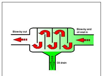
Figure 10: A simple labyrinth oil separator.
