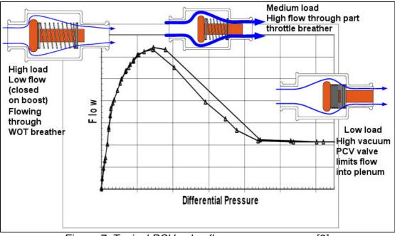
Figure 7: Typical PCV valve flow versus pressure [3].
