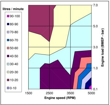
Figure 3: Blow-by volume map for a normally aspirated 1.6 litre gasoline engine
