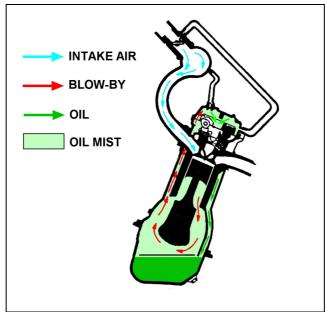
Figure 8: Oil mist and oil return circuit.
